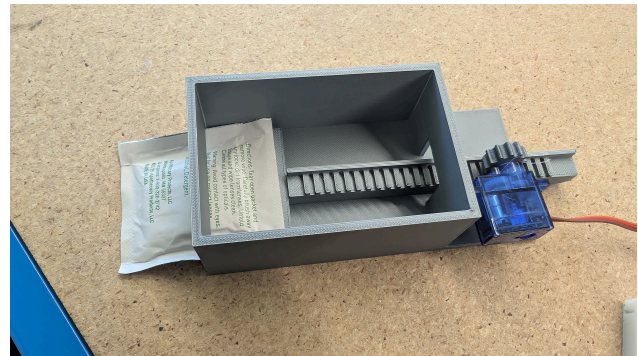
Figure 16: Mechanical dispensing test of Cartridge 2, showing the pusher sled driving an alcohol prep pad through the 2.5mm exit threshold.
